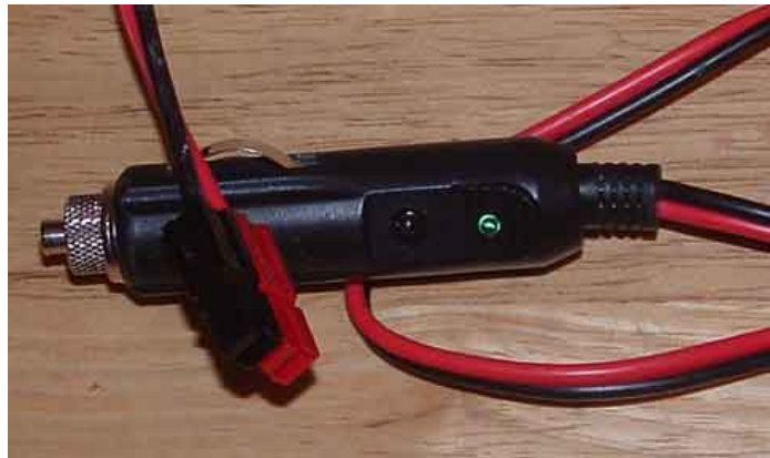
Figure 21 Because every cable created can be attached to the power distribution panel feeding power in, or out as needed allowing us to store or produce power, or consume power to and from the battery/charge controller package. I also wanted to power the radio from vehicles I made a cable that I can plug into a cigarette-lighter socket. Of course, all of these cables have multiple uses as they can be used in several different configurations linking the battery/controller or the solar panel to whatever device needs power, as the situation requires.
