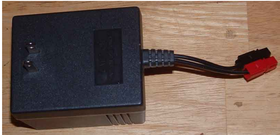
Figure 20 I cut the power cable a few inches from the potted adapter and crimped on the Andersen power-pole connectors. This would be when I'm on commercial power or where inverting AC is feasible. This power supply was perfect for powering my Yaesu FRG-100 shortwave receiver when AC power is available.
